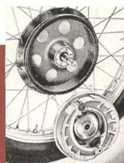
The new 8-in. front brake with super-ribbed shoes for smooth, efficient, straightline stops.
